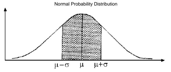
A normal distribution can be assumed when an uncertainty is quoted with a given confidence level. For example, a calibration report states that the uncertainty of a voltmeter is  $\pm$  0.1 V with a confidence level of 95%. The standard uncertainty of the voltmeter is given by:
