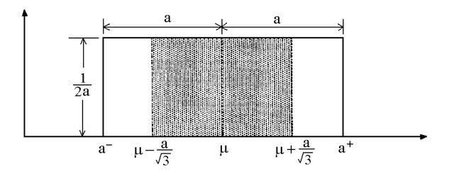
When an uncertainty is given by maximum bound within which all values are equally probable, the rectangular distribution can be assumed. For example, the accuracy of a voltmeter of a specific range is quoted as  $\pm$  0.2 V. The standard uncertainty of the voltmeter is given by:
